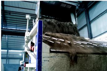
(3) Targeted fractionation of mineral construction waste: Highly contaminated material is separated from less contaminated material, so that many substances can be disposed of directly on site.
